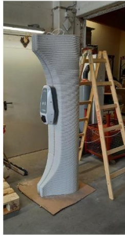
Figure 10: Prototype with AC Wallbox
